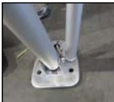
Align the ends of the Visor frame with the frame end point inserted into the small hole adjacent to the Dome leg on foot plate, repeating on both sides.
